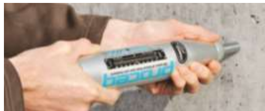
Figure 3. Schmidt hammer test.
